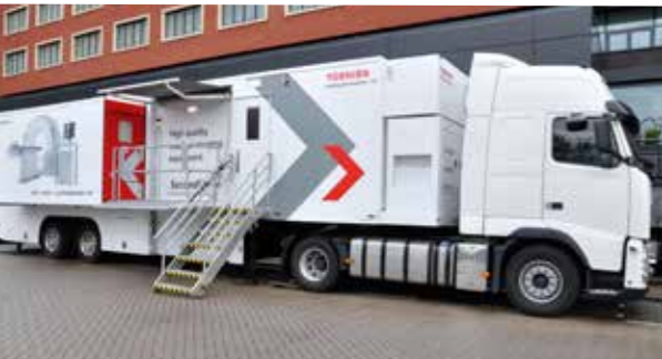
Refurbished CT system operated as a mobile system. (TMSE)
