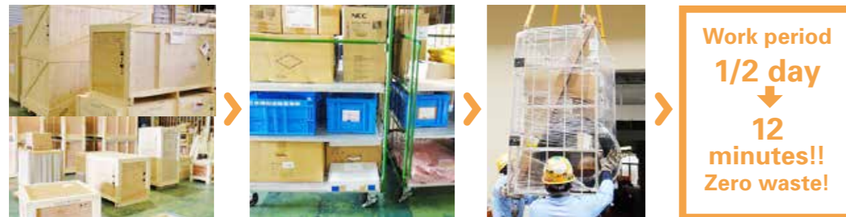
Products that were packed in conventional wooden frames are now arranged in an organized manner using a 3-level rack, and the products are shipped in place on the rack.
