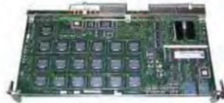
"Lead-free solder" (first used in PWBs for CT systems)
