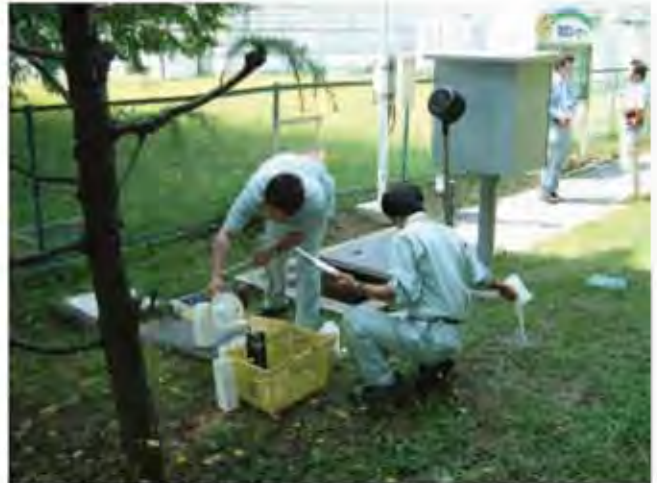
Sampling water at the final discharge outlet by the administration (every 3 months)
