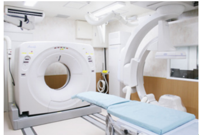
TMSC's X-ray angiography system combined with a self-propelled X-ray CT scanner installed at the Gate Tower Institute for Image Guided Therapy
