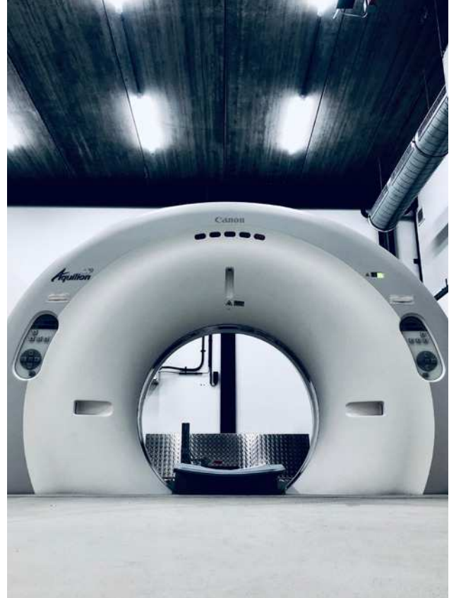
The platform and the gantry in a low position.
