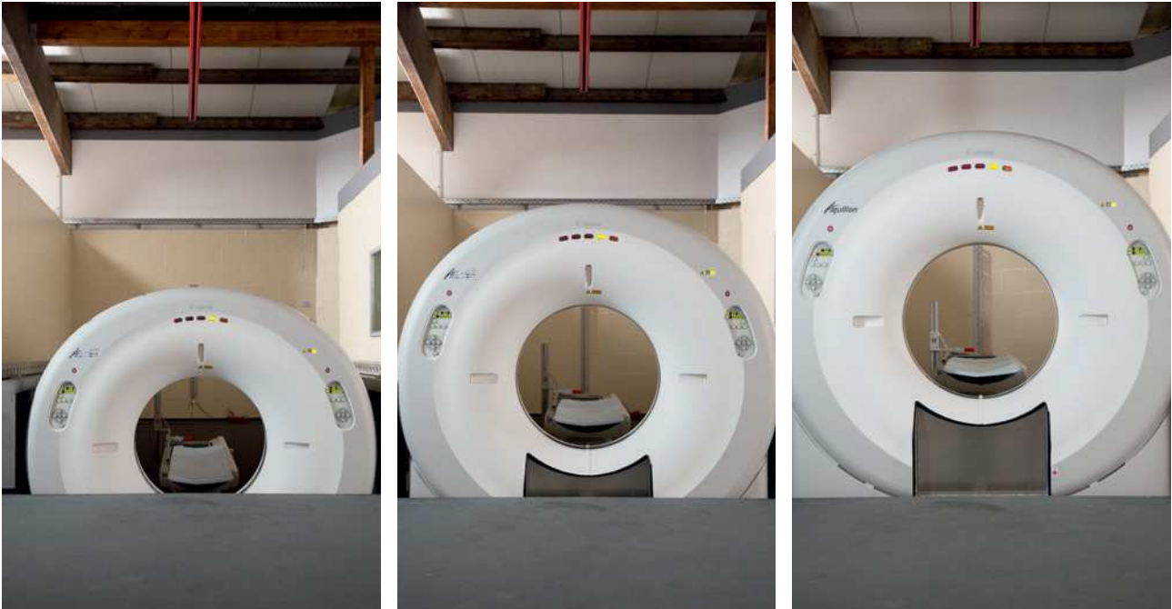
Height-Adjustable, Sliding Gantry CT System. First installations in Belgium, Germany and Switzerland. Photo: Bosdreef Referral Hospital for Horses
